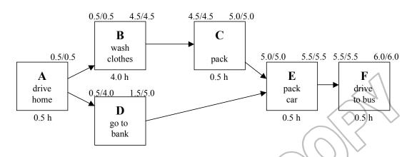
The final calculation is to identify the "slack" or "float" for each activity. Total slack is the maximum amount of time that an activity can begin late or be extended by, without delaying completion of the entire project. Notice that the slack time for an activity is <u>not</u> independent of the slack for other activities. Thus, it is <u>not</u> meaningful to add together the slack times of two or more activities.
