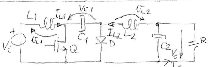
$$a) V_i \cdot DT = (V_{C1a} + V_D - V_i)(1-D)T \Rightarrow V_i \cdot D = V_{C1a} + V_D - V_i - V_{C1a} \cdot D - V_D \cdot D + V_i \cdot D \\ - V_{C1a}(1-D) = V_D(1-D) - V_i$$
