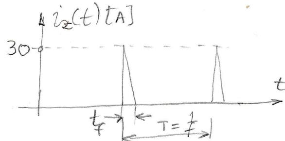
$$I_{Q\max} = \frac{\int_{0}^{t_f} V_p(t) dt}{L_p} = \frac{(V_z - V_i) t_f}{L_p} \Rightarrow t_f = \frac{I_{Q\max} \cdot L_p}{V_z - V_i}$$
