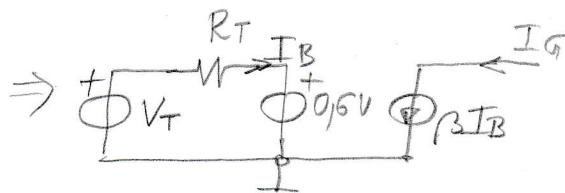
$$V_T = \frac{R_2}{R_1 + R_2} \cdot 12 = 2,863 \text{ V}$$
