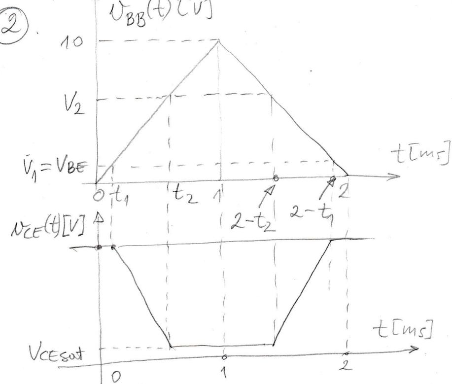
$$V_{CESat} = 12 - R_2 \beta I_{B2} \Rightarrow I_{B2} = \frac{12 - V_{CESat}}{\beta R_2} = \frac{12 - 0,2}{150 \cdot 10^3} = 78,7 \mu\text{A}$$
