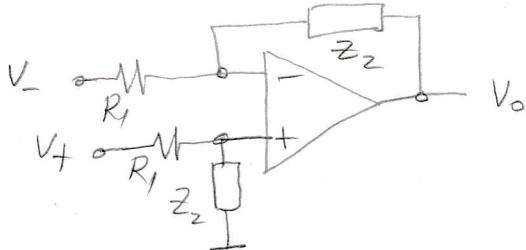
$$\Rightarrow V_o = (V_+ - V_-) \frac{z_2}{R_1}$$
