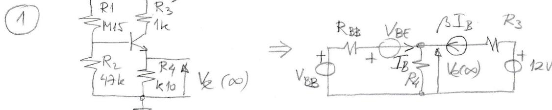
$$V_{BB} = \frac{R_2}{R_1 + R_2} \cdot 12 = \frac{47}{150+47} \cdot 12 = 2,86 \text{ V} ; \quad R_{BB} = R_1 // R_2 = \frac{150 \cdot 47}{150+47} = 35,8 \text{ k}\Omega$$
